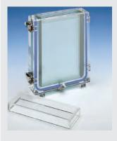
Both the GCC-404K (4-place) and the GCC-410K (10-place) Casting Chambers fit all 16.5cm wide glass plates with heights up to 22cm. Each kit includes:
